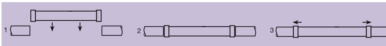
Figure 6-2 Closure section assembly
